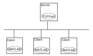
You use the same basic network installation procedure to install MathWorks products on a client computer. The installation documentation notes any differences between the installations.
